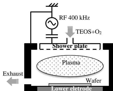
Fig. 1. Schematic view of PECVD.
