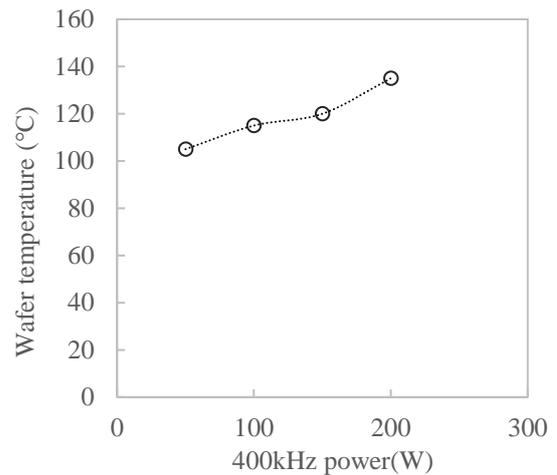
Fig. 4. Variation of wafer temperature as a function of 400kHz power.
