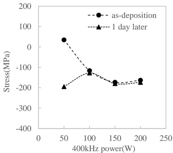
Fig. 2. Variation of Stress as a function of 400kHz power.
