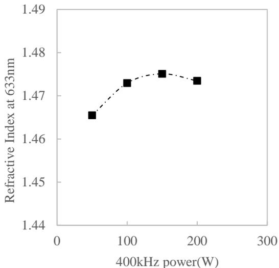
Fig. 3. Variation of refractive index as a function of 400kHz power.
