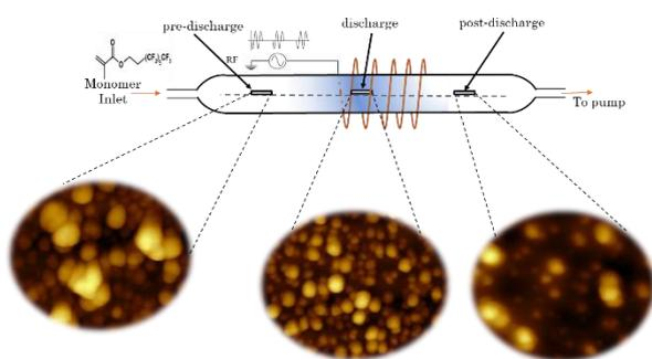
Fig.1. Schematic illustration of the low-pressure plasma reactor used for this study. The different studied positions of the sample are indicated (pre-discharge, discharge and post-discharge) and the AFM images of coating surfaces obtained at each discharge position are illustrated.
