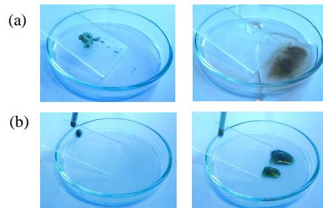
Fig. 6. (a) Self-cleaning processes for the PFAC coated glass surface. (b) Resistance to muddy water drops for the coated glass surface in antifouling tests.
