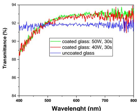
Fig. 7. Direct optical transmission of uncoated and coated glass as a function of wavelength.
