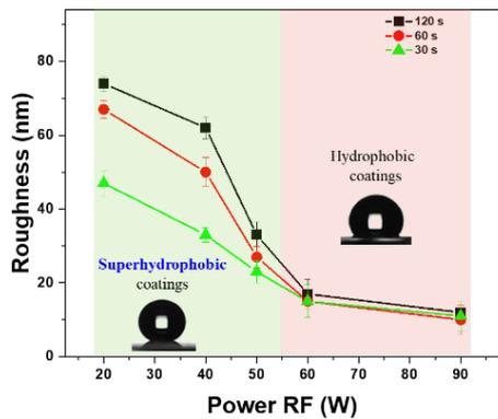
Fig. 4. Roughness of PFAC coatings plasma as a function of power RF and deposition time. Inset: Digital photograph of water liquid droplet on the plasma coating.
