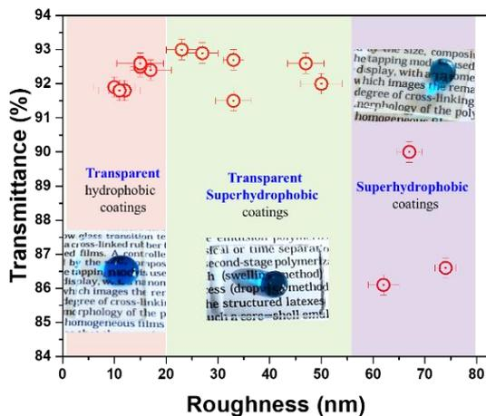
Fig. 5. Transmittance vs roughness of PFAC coatings plasma. Inset: Optical photos of methylene blue dyed water droplets on coated glass substrate.
