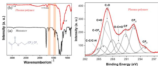
Fig. 2. Infrared spectra of 1H,1H,2H,2H-perfluorooctyl acrylate (left): (a) monomer; (b) PFAC plasma coating. XPS high-resolution spectra of C(1s) of PFAC coating (right).
