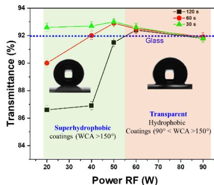
Fig. 3. Transmittance ( $\lambda = 600 \text{ nm}$ ) of PFAC coatings plasma as a function of power RF and deposition time. Inset: Digital photograph of water liquid droplet on the plasma coating.
