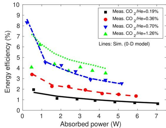
Fig. 3. Energy efficiency of a RF He/CO<sub>2</sub> plasma jet. The measurement data (points) are taken from [3]. The simulation results (lines) are from this study.
