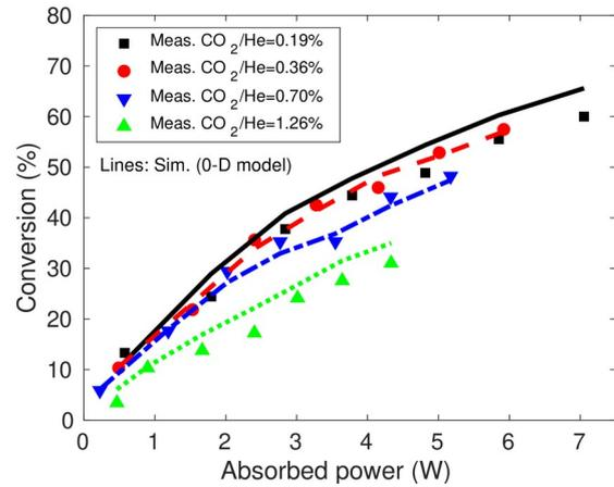
Fig. 2. Conversion efficiency of a RF He/CO<sub>2</sub> plasma jet. The measurement data (points) are taken from [3]. The simulation results (lines) are from this study.
