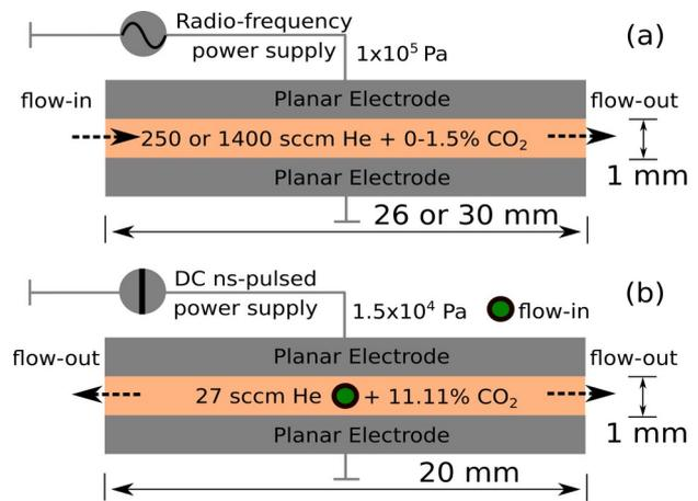
Fig. 1. Sketch of plasma jet chambers
