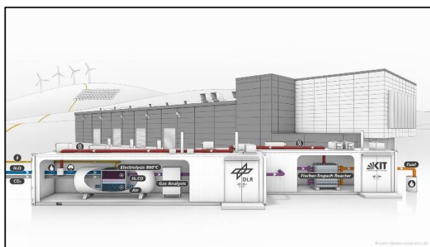
Fig. 1. Sketch of the e-XPlore transportable research platform, which is jointly provided and operated by KIT and DLR
