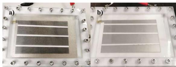
Fig. 1. a) grid electrodes with phlogopite. b) plate electrodes with ceramic dielectric.
