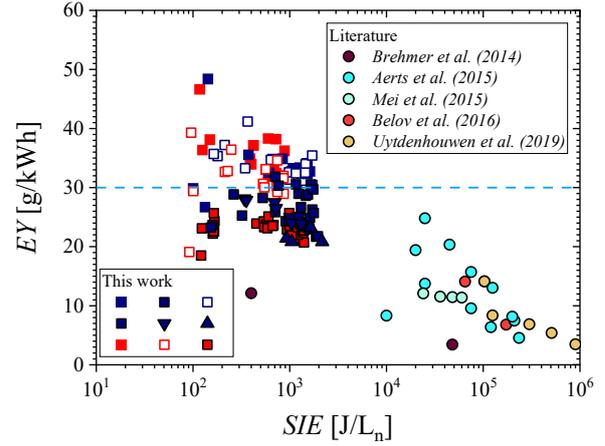
Fig. 3. Energy yield of CO formation as a function of  $SIE$  for the different DBD reactors.
