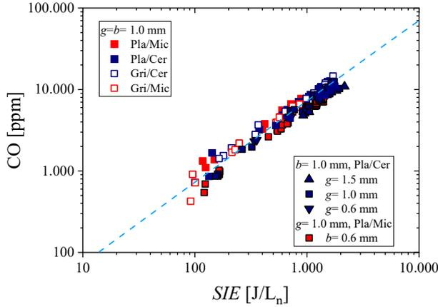
Fig. 2. CO fraction as a function of  $SIE$  in the different reactor configurations. The colors represent the dielectric, full symbols are for plate electrodes, open symbols are for grid electrodes.
