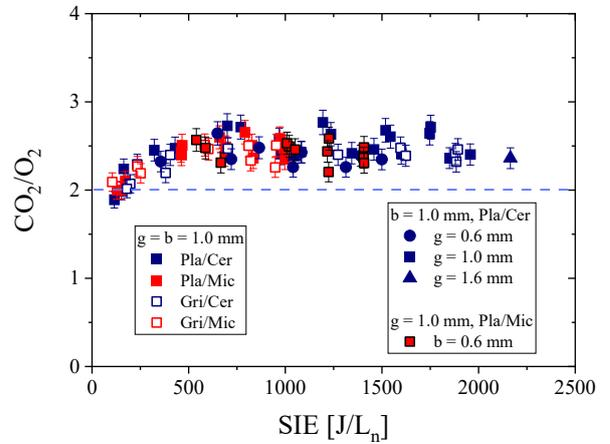
Fig. 4. Stoichiometric ratio considering only molecular oxygen for the balance in the different DBD reactors.
