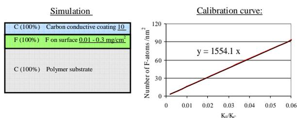
Fig. 3 Determination of K-ratios ( $K_F/K_C$ ) with simulation STRATAgem varying the area density of F atoms from 3.2 up to 96  $\text{per nm}^2$ .
