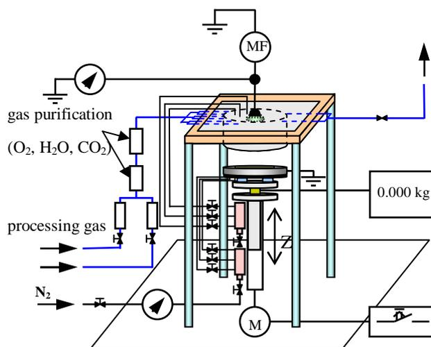
Fig. 1 Setup for plasma printing of amino groups.
