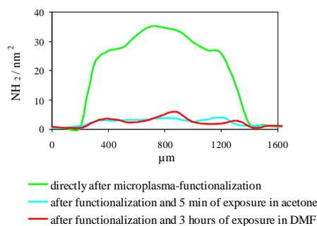
**Fig. 5** Distributions of primary amino group densities across the diameters of plasma-printed 1000  $\mu\text{m}$  spots on PP/C204 composite obtained in  $\text{N}_2 + 4\% \text{H}_2$  at 10 s of microplasma-treatment duration.
