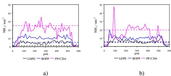
**Fig. 4** Distributions of primary amino group densities across the diameters of plasma-printed 500  $\mu\text{m}$  spots on LDPE, BOPP, and PP/C204 composite, resp., obtained (a) in  $\text{N}_2 + 4\% \text{H}_2$  and (b) in  $\text{N}_2 + 10\% \text{NH}_3$  by CD SEM-EDX. Average values calculated from CD ATR-FTIR measurements are shown for comparison as dotted lines.
