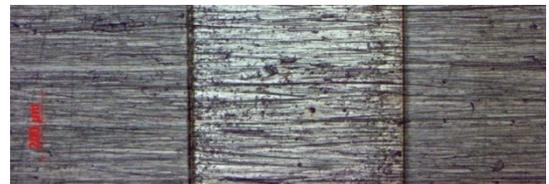
Fig. 5: 100-times magnified microscope picture of by laser and plasma ablated area, fluence 1.0  $\text{J}/\text{cm}^2$
