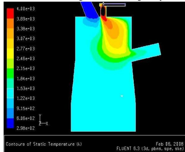
Fig. 1. Temperature distribution in the reactor (global view) (Range 298 K – 4000 K)
