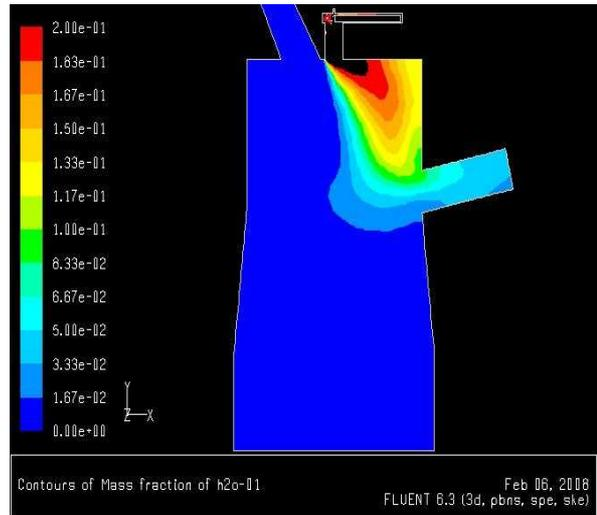
Fig. 4. Contours of mass fraction of steam
