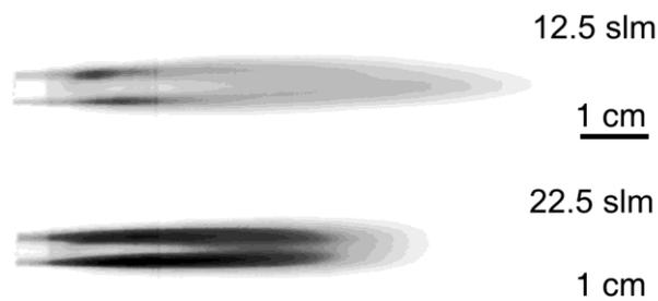
Fig.1 Structure of plasma flow at different argon flow rates (12.5 and 22.5 slm). Darker color means higher intensity of fluctuation of plasma radiation.
