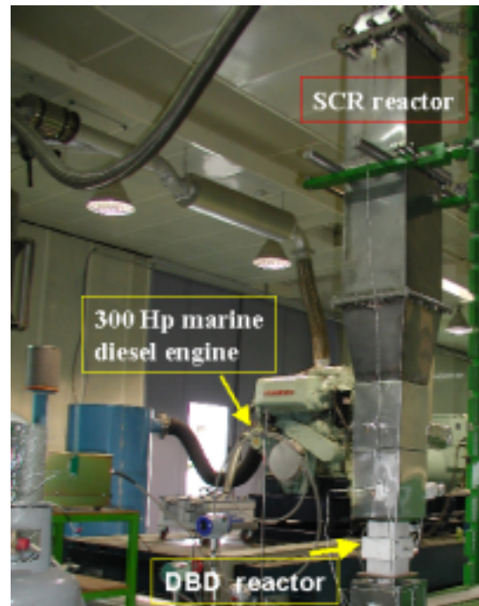
Fig. 3 Pilot-scale plasma/SCR combined system with marine diesel engine.
