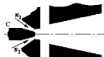
Fig. 1 Layout of the plasmatron with expanding channel of the outlet electrode (C – cathode, A – anode, I – insulating insertion).
