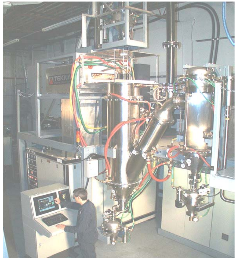
Figure 1: A 200 kW industrial unit of powder spheroidization, manufactured in Tekna Plasma Systems. This system produces spheroidized cemented powders at the productivity of 30 kg/h.
