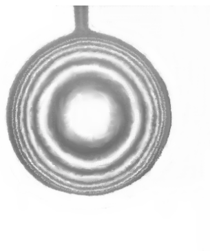
Fig. 6. Optical interferogram of glass shell received by displacement interferometer. On surface of glass microsphere the layer of plasmochemical silicon dioxide is put. Common thickness of wall together with a covering is 11 microns.
