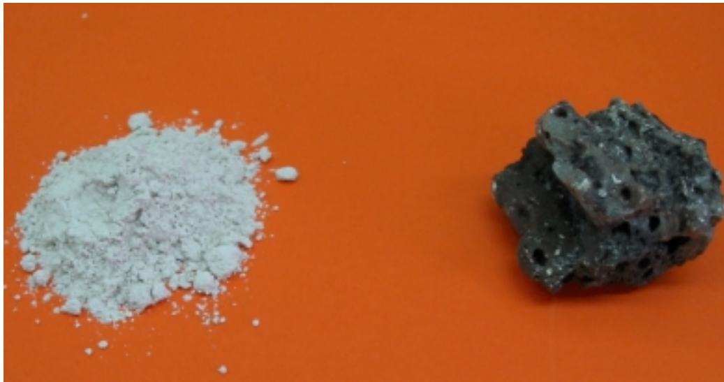
Fig.2. Starting fly ash (left) and the plasma melted product (right)
