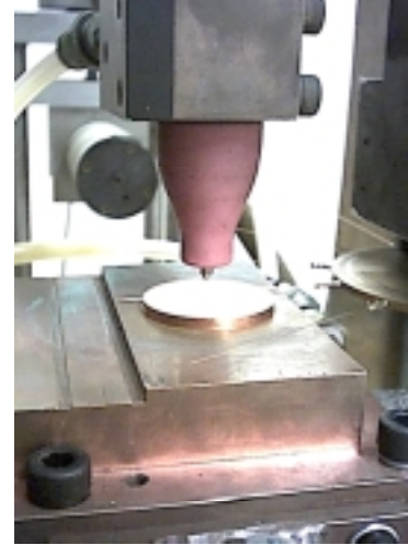
Figure 2, setup for the Langmuir probe. The probe disk sweeps probes through the arc (in between cathode and anode shown in orange). Right, torch nozzle with W tip, and copper anode. A portion of the multi probe disk with protruding probes is shown
