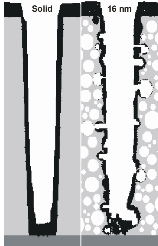
Figure 6 – High Aspect Ratio features (solid SiO 2 and 16 nm PS) lined with copper following IMPVD. The dark material on SiO 2 is copper. Presence of pores creates or initiates voids. This effect is pronounced for larger pores.
