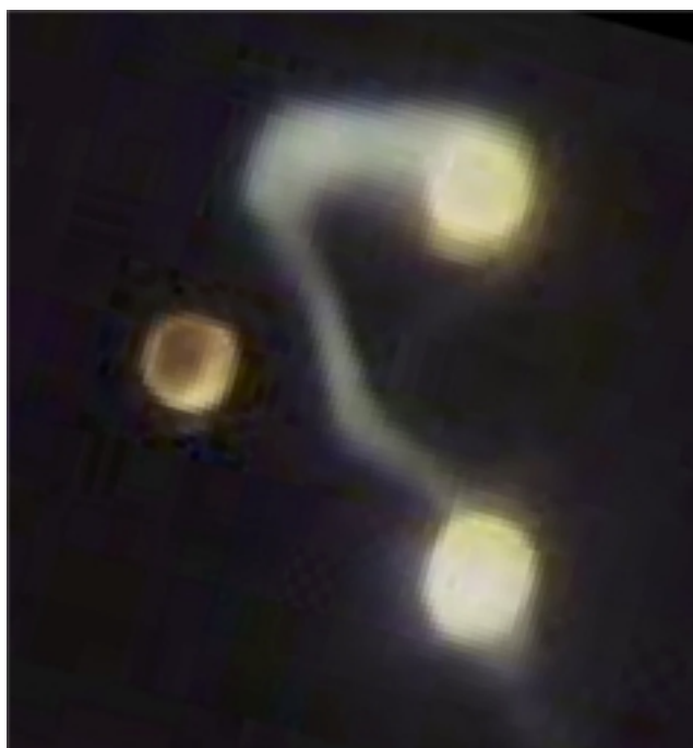
Figure 2. Arc view from the bottom of the reactor (plane XY ) obtained by ultrahigh-speed cine-camera in argon plasma.
