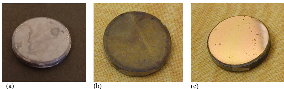
Figure 2 - Silver-base alloy samples (Ag90Cu10) after 24h of immersion in 0.1M \text{Na}_2\text{S} : (a) uncoated; (b) coated with 900 nm PECVD \text{SiO}_x -like film (TEOS 3 sccm, \text{O}_2 50 sccm, Ar 36 sccm, at 200W); (c) coated after \text{H}_2 -plasma treatment
