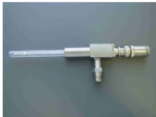
Figure 2: Plasma torch (right – rf connection, down – helium inlet).
