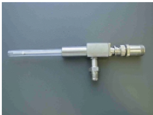
Figure 2: The plasma needle used for tissue treatment: left – helium-filled moveable plastic tube surrounding the needle, down – helium inlet, right – rf connection.
