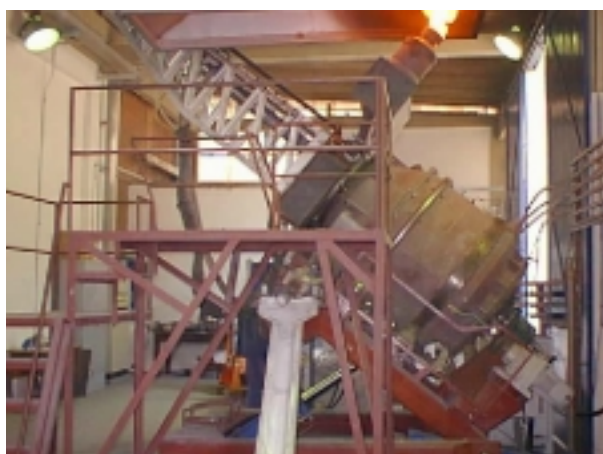
Fig. 1 – Overview of plasma heated Al recovery furnace, 300 kg capacity.
