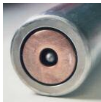
Figure 2 : Details of plasma gas injection
