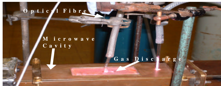
Figure 3: Experimental setup for optical measurements
