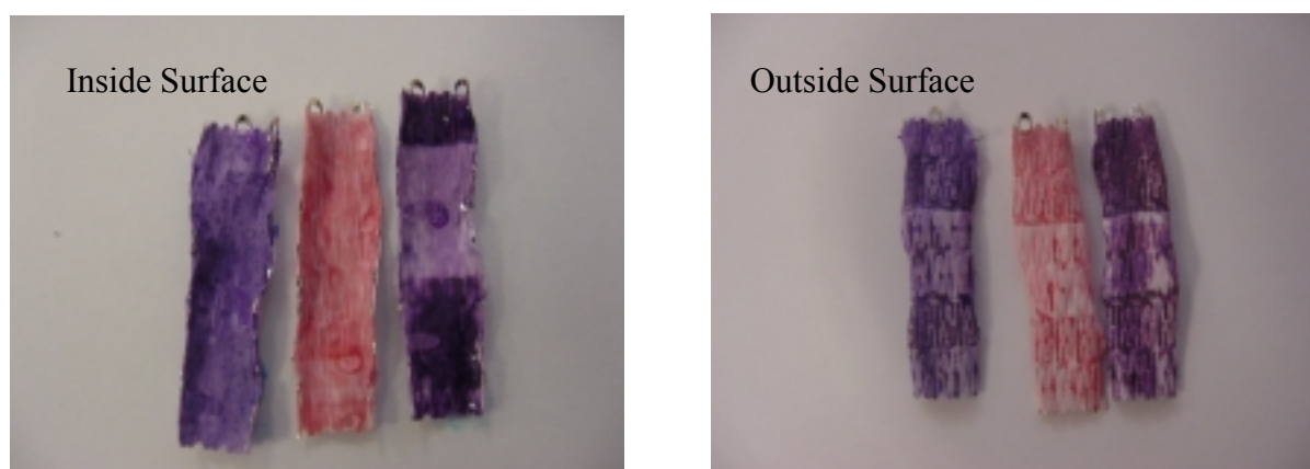
Fig. 3 Results of staining tests showing the effect of the presence of the plasma-deposited layer on the yield of the graft-coupling reaction. The photograph shows test samples after (left to right) acrylic acid grafting, anionic surface, toluidine blue stain; PEI coupling, cationic surface, Ponceau S stain; heparin coupling, anionic surface, toluidine blue stain. (VCOAT is the trademark of the heparin coating). Samples were cut and flattened to show the whole surface.
