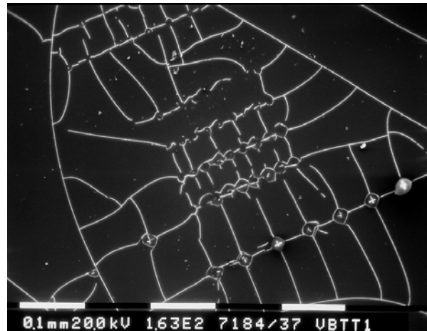
Fig. 2 SEM image of the crack network developed around the matrix of indentation prints.
