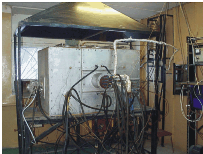
Fig. 2. Pilot plant for waste destruction based on the new plasma chemical reactor.
