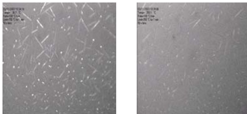
Fig.5 Comparison of thermal stability of observable nanotubes polymer slices through polarization micrographs at different testing temperatures
