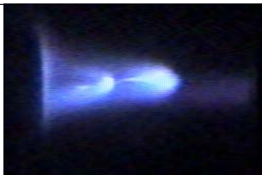
Fig. 9. The luminescence of dispersed kerosene in the trans-sonic air-EBP flow; the mixture isn't ignited.
