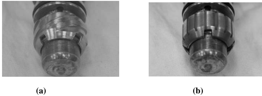
Fig.2 Plasma gas feeding guide (a) for swirling flow and (b) for straight flow.
