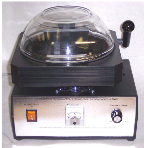
Fig. 5: a) An universal plasma reactor UPS100W.
