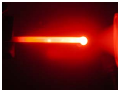
Fig. 1: Plasma heating of a ceramic sample
