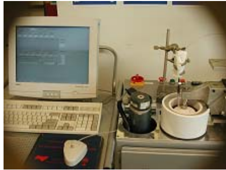
Figure1- The pin-on-disc wear testing machine used.
