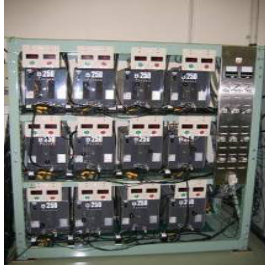
Fig. 3 Setup of the twelve-phase AC power supply
