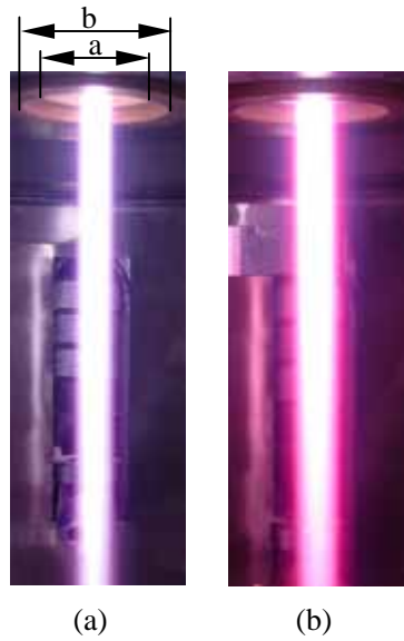
Fig. 2 Photographs showing the appearance of the pure argon (a) and Ar-H 2 (b) laminar plasma jets. Sizes a and b are 60 and 76 mm, respectively, representing the inner and outer diameters of anode flange plate.
