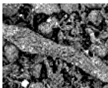
Figure 3b. Air plasma treated \kappa -carrageenan at 125W for 20 min (X500)
