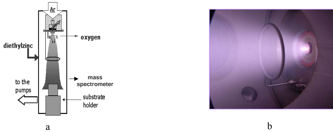
Figure 1. a) Schematic of the deposition reactor; b) Argon expanding thermal plasma ( \Phi_{Ar} = 1000 sccm, p_{chamber} = 0.3 mbar); the O 2 ring and the arc nozzle are visible.
