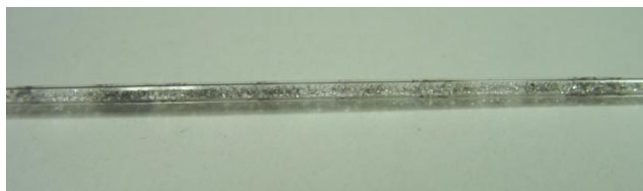
Fig. 7 The photograph of the capillary packed with glass beads and the deposited thin film including palladium at the substrate temperature of 130 °C.
