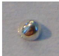
Fig. 4. The final experimental tin splat morphology - (a), at KPPs: D_p=1.55 mm, u_{p0}=0.75 m/sec, T_{p0}=535 K, T_{b0}=290 K; the numerically predicted spreading and solidifying droplet at time moments 2 msec, - (b), and 9 msec - (c). We=11 , Pe=67 , Re=4381 .
