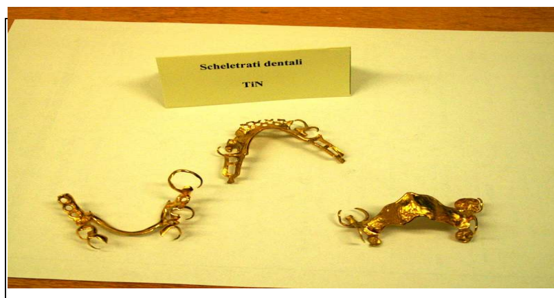
Fig.3. Images of different typical dental materials prostheses with complex geometry coated with TiN
