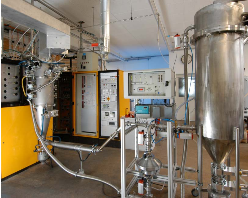
Figure 1: Photograph of the inductively coupled plasma (ICP) equipment for nanoparticle synthesis.
