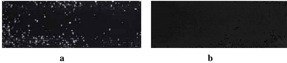
Fig.9 Ink printability on UV cured resin a-before and b-after DBD gun treatment
