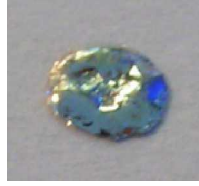
Fig. 6. The final experimental tin splat morphology - (a), at KPPs: D_p=1.55 mm, u_{p0}=1.64 m/sec, T_{p0}=528 K, T_{b0}=290 K; the numerically predicted spreading and solidifying droplet at time moments 1 msec - (b), and 2 msec - (c). We=54 , Pe=147 , Re=9603 .
