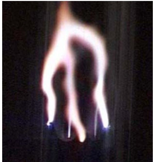
Fig. 4. a), b) Courses of voltage and current of the gliding discharge in two and three electrode reactor, respectively, c) side view of the discharge
