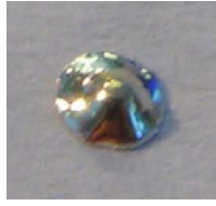
Fig. 5. The final experimental tin splat morphology - (a), at KPPs: D_p=1.55 mm, u_{p0}=1.16 m/sec, T_{p0}=532 K, T_{b0}=290 K; the numerically predicted spreading and solidifying droplet at time moments 2 msec - (b), and 4 msec - (c). We=27 , Pe=104 , Re=6772 .
