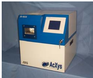
Figure 6 : Bench-top plasma system for batch treatment of small objects.
