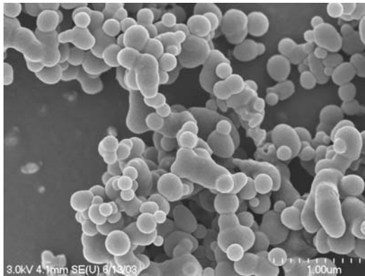
Figure 3: SEM micrographs of the plasma synthesized powders: ( \text{La}_{0.8}\text{Sr}_{0.2}\text{MnO}_{3-\delta} )
