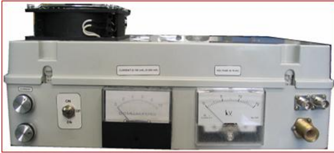
Figure 9: Reactive Capacitive Resistance based power supply, specially developed for GA's
