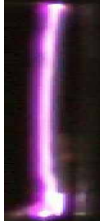
Fig. 2a. Colorized arc photo (arc current 0.7A, magnetic field 0.8T)
