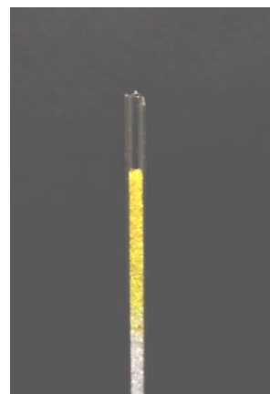
Fig. 8 Silica gel particles adsorbed by \text{Pd(hfac)}_2 .
