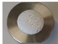
Martindale abrasion test
