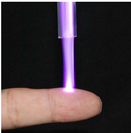
Fig.2 LF plasmajet exhausted to a finger without burning.
