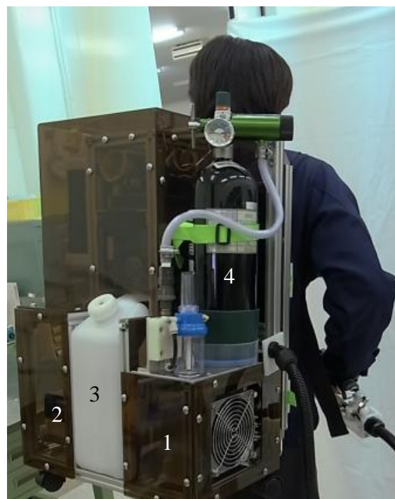
Fig.1 A portable ozone mist system 1. Ozone generator 2. DC-AC inverter 3. Water container 4. Oxygen cylinder
