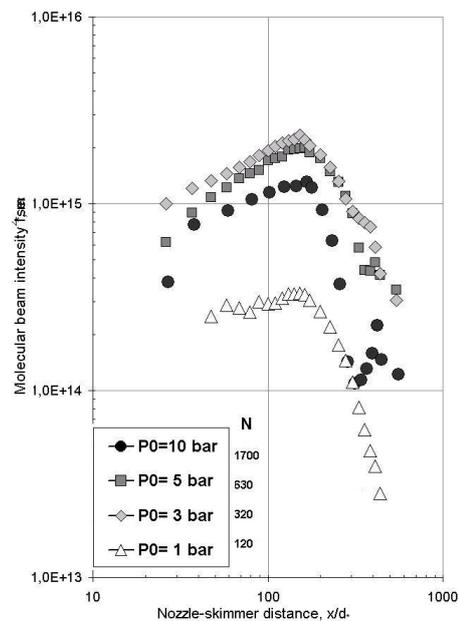
Fig.3. Cluster beam intensity dependence of nozzle-skimmer distance.
