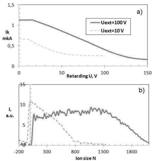
Fig.4.a. Ion current dependence of retarding voltage.
