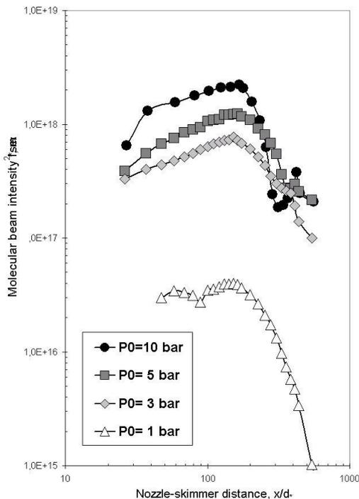
Fig.2. Molecular beam intensity dependence of nozzle-skimmer distance.
