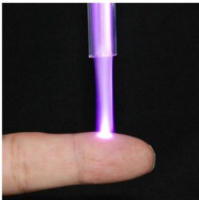
Fig.1 LF plasmajet exposed to a finger without burning.
