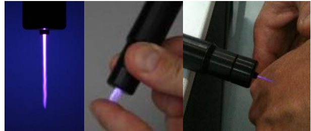
Fig.1 Dual gas nanosecond pulsed plasma jet with He (left and right) and Ar (center) as primary gas
