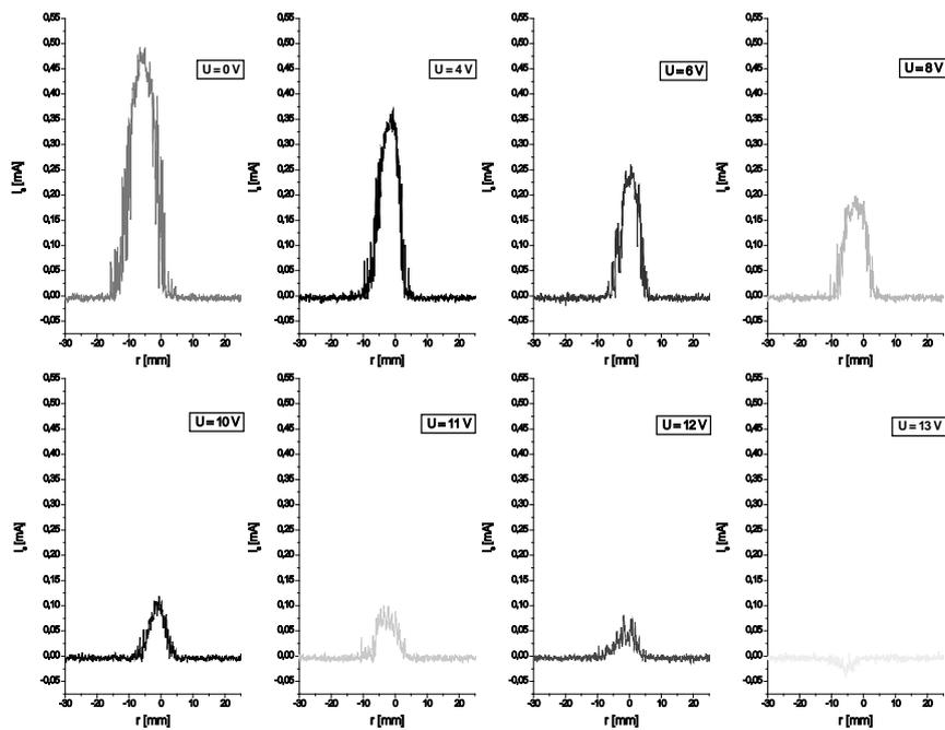
Fig. 2. Probe currents for various values of biasing voltage ( $I = 200$  A, argon flow rate 12.5 slm, chamber pressure  $P = 30$  kPa, axial distance from plasma torch 100 mm)
