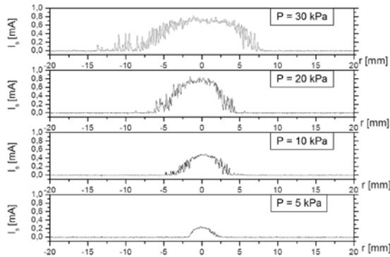
Fig. 4. Probe currents for biasing voltage  $U = 0$  V for various ambient pressures. Axial position 100 mm.
