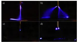
Fig. 2. Photos of air corona discharges applied on glass cover slides, first row is PC a) without electrospray with sharp needle, b) electrospray with clipped needle. Second row is NC c) sharp needle, d) clipped needle with electrospray.
