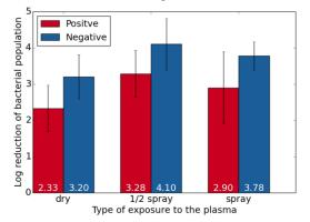
Fig. 3. Logarithmic reduction of bacterial population for three different exposure conditions to corona discharges (3-5 replicates, mean±SD).
