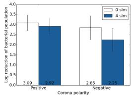
Fig. 4. Logarithmic reduction of bacterial population by the corona discharges with or without blowing of air through the discharge, exposure time  $5 \min (5-8 \text{ repeats}, \text{mean}\pm\text{SD})$ .
