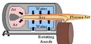
Fig. 1. Schema of the argon/water DC plasma torch.
