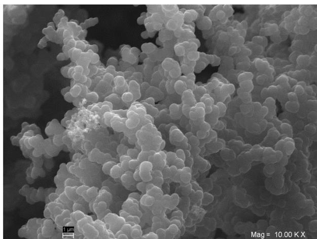
Fig. 5. Carbon black particles, sampling position B, particle size 400 - 1000 nm.
