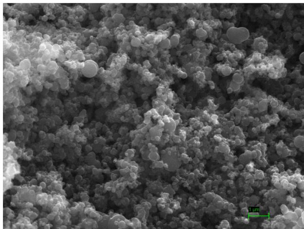
Fig. 4. Carbon black particles, sampling position A, particle size 100 - 800 nm.
