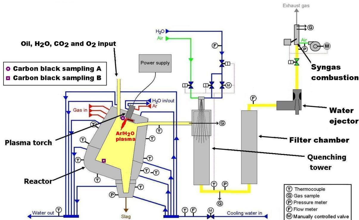
Fig. 2. Schema of experimental reactor.
