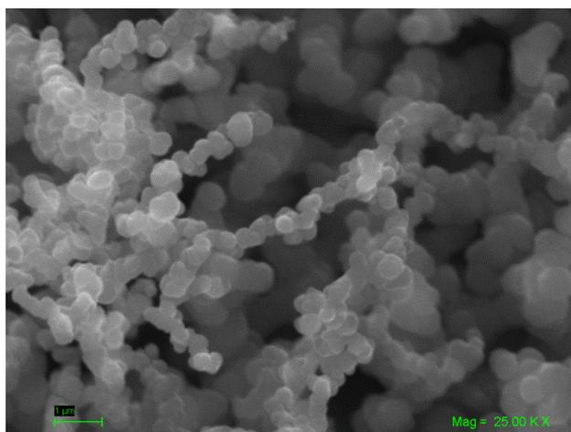
Fig. 6. Carbon black particles, sampling position B, particle size 180 - 600 nm.
