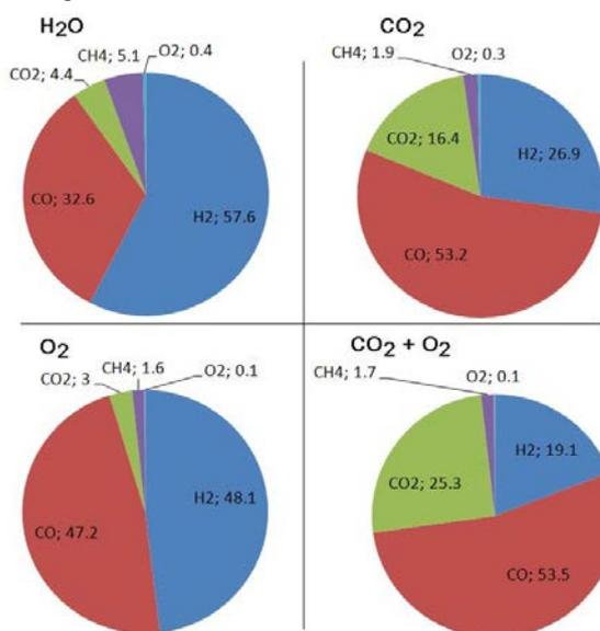
Fig. 3. Gas compositions of syngas for different types of oxidation (values in vol. %).
