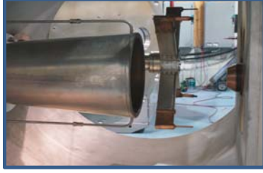
Fig. 2. Catch cone and rotary arm with probes for plasma plume and material characterization
