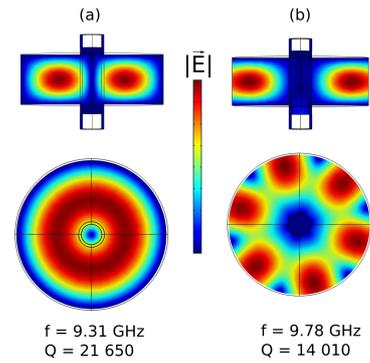
Fig. 3. The comparison of EM fields (rz-plane) and Q-factors for two computed modes around 9.3 GHz (the one on the left (a) being the used  $TE_{110}$  mode).
