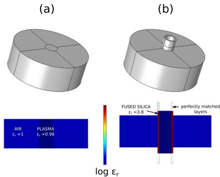
Fig. 2. The (a) simple and (b) advanced model geometry with colour coded permittivity shown in the rz-plane.
