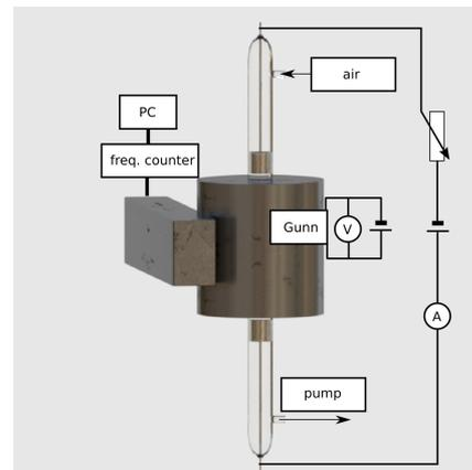
Fig. 1. The cylindrical microwave resonator set-up.
