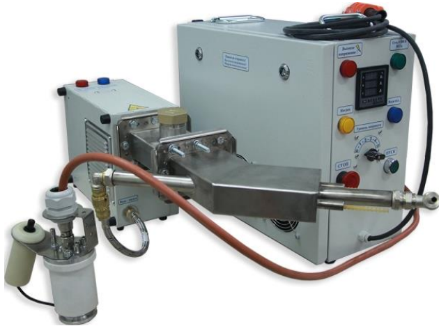
Fig. 2. The general view of universal hardware complex for obtaining of low-temperature and ANT plasma.
