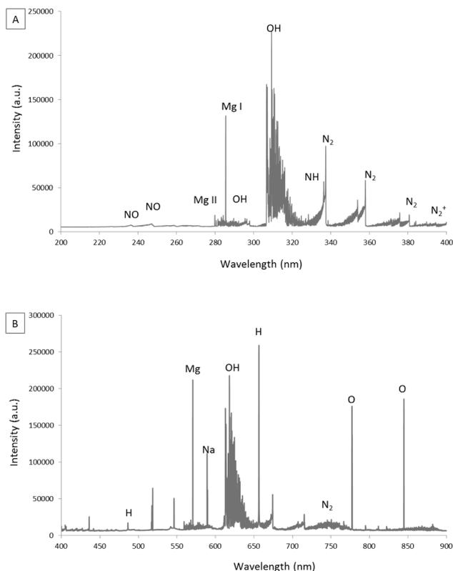
Fig. 2. OES spectra acquired during synthesis of PAL.
