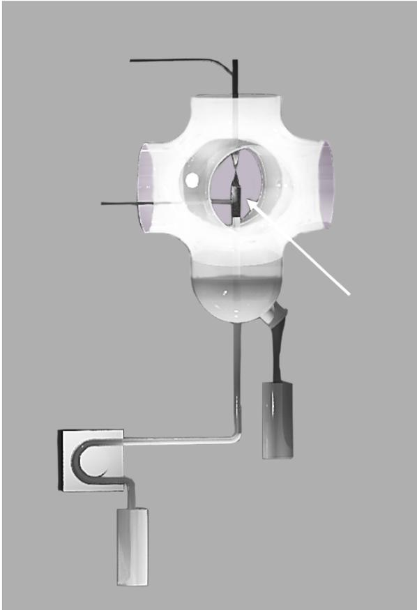
Fig. 1. A schematic representation of dc-APGD-based reaction-discharge system for the continuous synthesis of PAL dedicated for eradication of *P. parmentieri*. The arrow shows dc-APGD, which is a type of CAPP.
