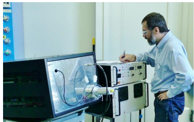
Fig. 1. Glassman High Voltage, Inc. 8 kW – 15 kV power supply and a home-made variable resistor box with a mounted high-voltage probe.
