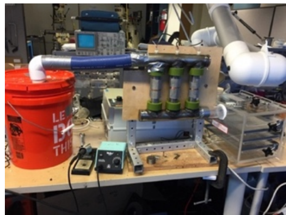
Fig 1. Photograph of the 2,500 in 3 DBD misting system
