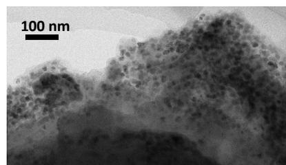
**Fig. 6** TEM bright field image of the GNP-embedded cross-linked gelatine thin film.
