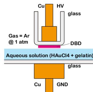
**Fig. 4** Schematic illustration of the experimental setup for thin film formation on liquid surface.
