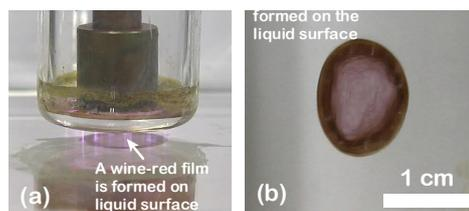
**Fig. 5** DBD on aqueous solution of HAuCl<sub>4</sub> and gelatine can create free-standing thin film composed of GNP and cross-linked gelatine.
