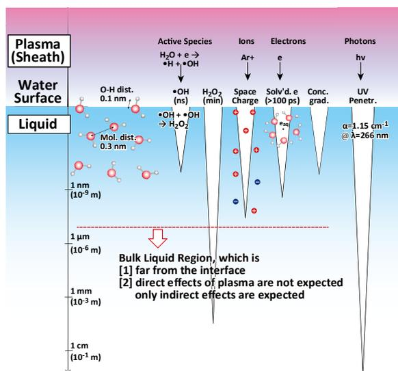
**Fig. 1** Schematic illustration of a water interface together with indication of the penetration depth of direct effects provided by plasma.
