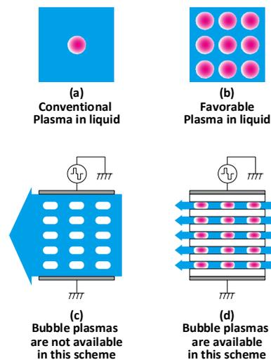
**Fig. 2** (a) Conventional plasma in liquid, (b) Favourable plasma in liquid, (c) Simple idea which does not work, (d) practical approach for realizing (c).
