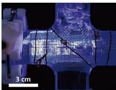
**Fig. 3** Overview of a 3D integrated micro solution plasma reactor constructed on the basis of concept (d) in Fig. 2.
