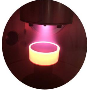
Fig. 2: Plasma expanded from the MHCD to the polarized heated silicon substrate.
