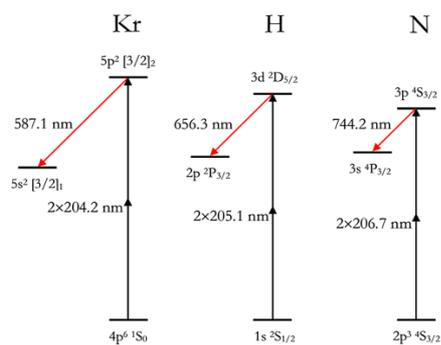
Fig. 2. Two-photons energy transitions schemes to perform TALIF measurements of H, N and Kr ground states.
