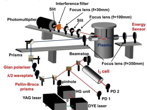
Fig. 1. Experimental arrangement deployed to perform TALIF measurements.
