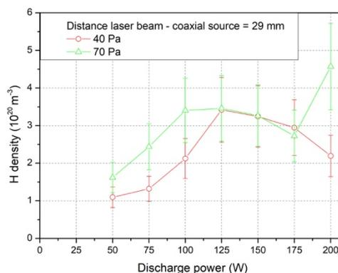
Fig. 4. Atomic Hydrogen density as a function of discharge power evaluating pressure effect at a fixed distance (29 mm) from coaxial source.
