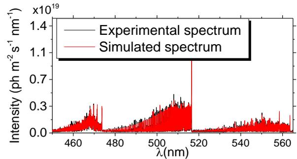
Fig 2. Typical emission from the  $C_2$  Swan band, data obtained at 900 W power and 10 slm  $CO_2$  flow.
