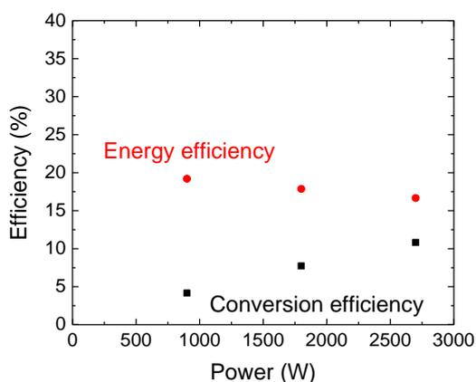
Fig 3. Energy efficiency and conversion efficiency measured at atmospheric pressure and 20 slm  $\text{CO}_2$  flow.
