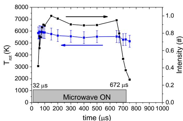
Fig 4. Typical  $\text{C}_2$  rotational temperature (in blue) and intensity (in black) behaviour during a pulse. Data acquired at peak power 2700 W, with 20 slm  $\text{CO}_2$  flow. Pulse frequency 1 kHz with a duty cycle of 65%.
