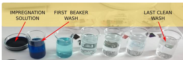
Fig. 2. Finding the optimum number of washing steps by methylene blue impregnation and set of washings.
