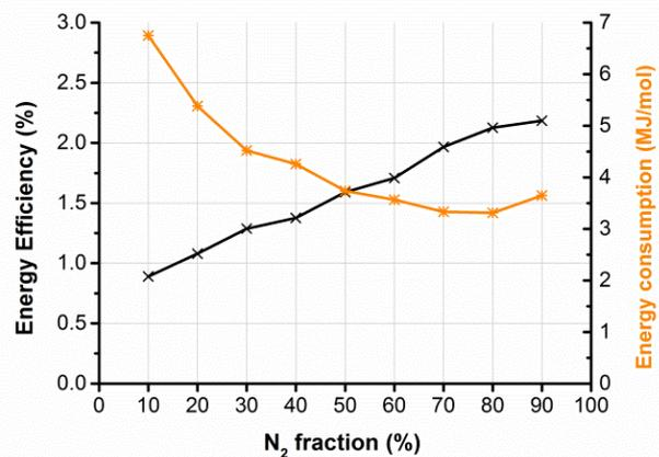
Fig. 5. Energy efficiency and energy consumption for different  $N_2$  fractions in the feed gas, at a total flow rate of 10 L/min.
