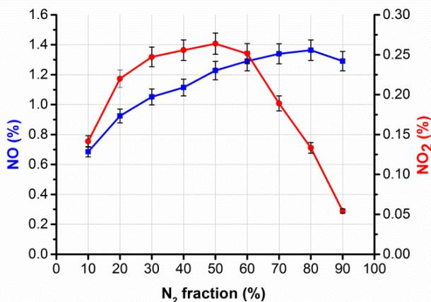
Fig. 3. Concentration of NO and  $NO_2$  for different  $N_2$  fractions in the feed gas, at a total flow rate of 10 L/min.
