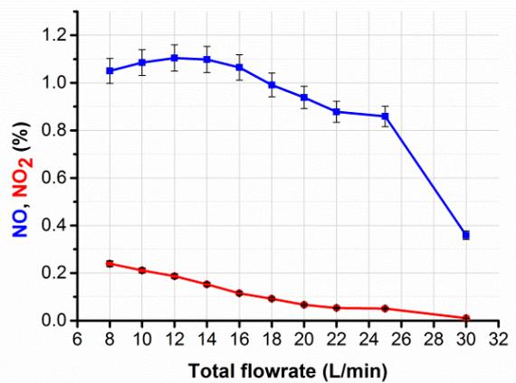
Fig. 4. Concentration of NO and  $NO_2$  at different total flow rates, with  $N_2$  fraction of 80%.
