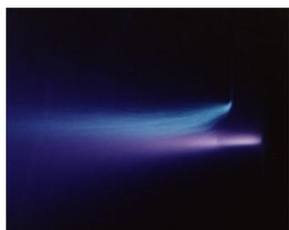
Fig. 5. The injection of chitosan solution into the EBP flow.
