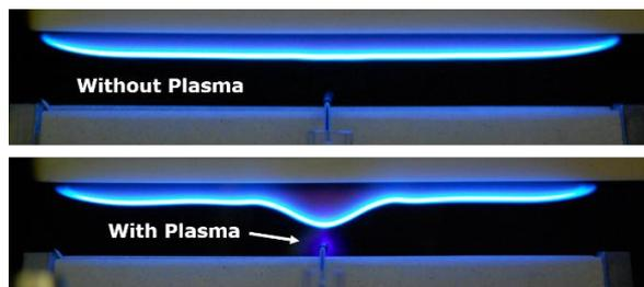
Fig. 1. Plasma-assisted flame in slot burner
