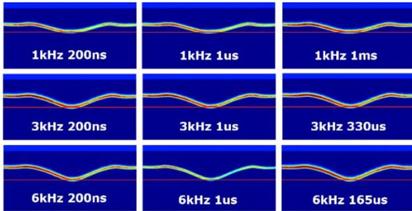
Fig. 3. Flame displacement for various PRF after 200 ns, 1  $\mu$ s and right before the following discharge
