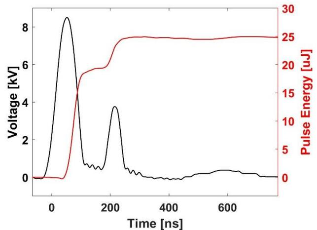
Fig. 2. Pulse voltage and pulse energy for a PRF of 1 kHz
