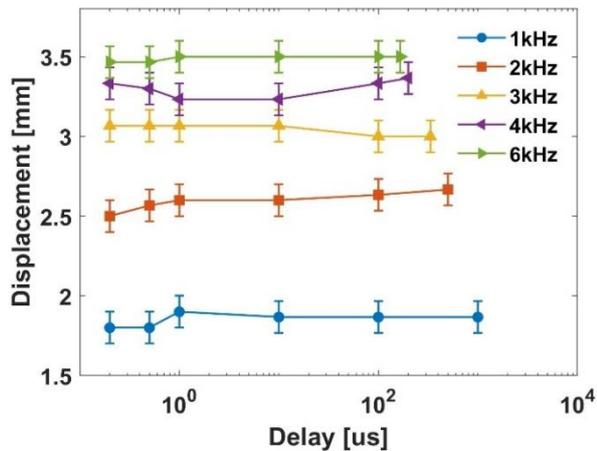
Fig. 4. Flame upstream displacement for various delays between two consecutive discharges
