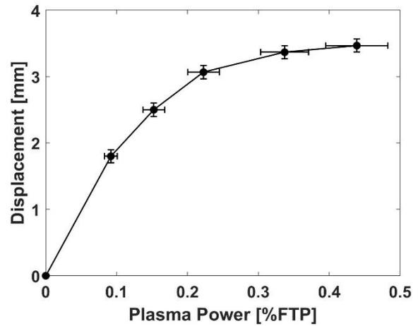
Fig. 5. Percentage of the flame thermal power (FTP) required to produce the observed displacement
