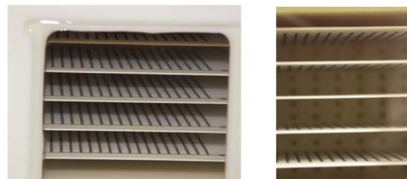
Fig. 2. Photograph of the reactor with 5 stacked symmetric SDBD electrodes.
