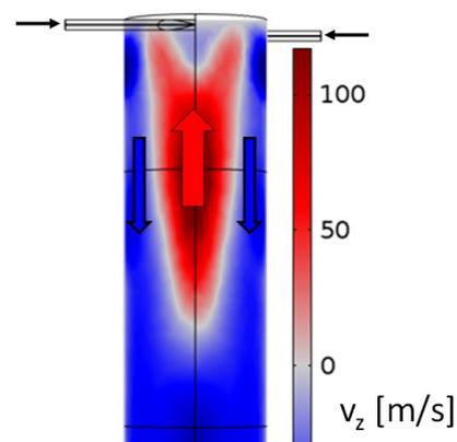
Fig. 1: Forward vortex flow - On-plane projection of the z-component of the gas flow
