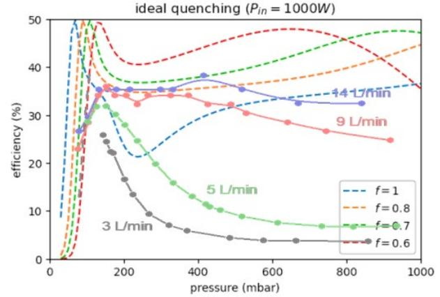
Fig. 4: Experimental efficiency values as function of pressure (dots) and the efficiency limitations obtained from the 2-temperature model (dashed lines)
