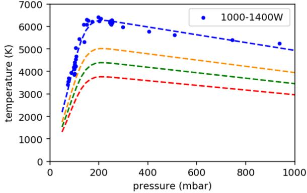
Fig. 3: Core gas temperature measurements as function of pressure. The dashed lines show temperature parameterizations of  $T_1$  in blue ( $f=1$ ), orange ( $f=0.8$ ), green ( $f=0.7$ ) and red ( $f=0.6$ ).
