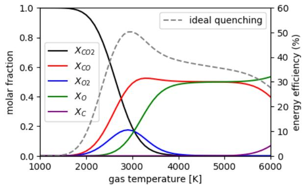
Fig. 2: Thermodynamic equilibrium calculation of the molar fractions and ideal quenching efficiency of CO<sub>2</sub> at a fixed pressure of 100 mbar, as function of temperature.
