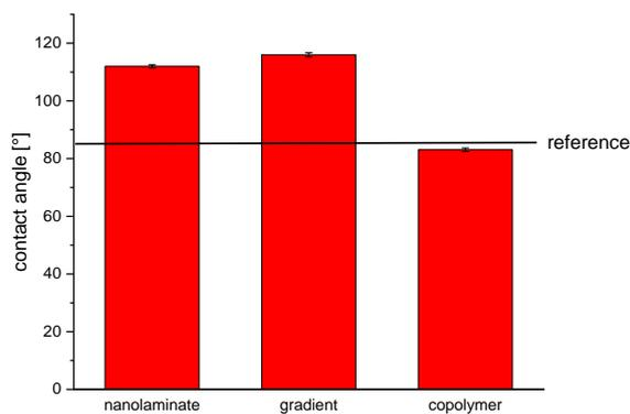
Fig. 3. Contact angle measurements on coated plates.
