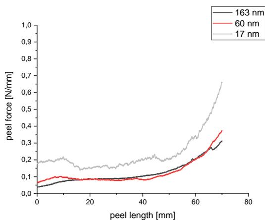
Fig. 6. Peel forces as a function of the thickness of the anti-sticking coating.
