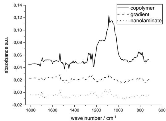
Fig. 4. Subtracted IR-spectra of laminated polymer foils after peel test.
