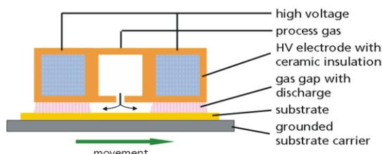
Fig. 1. Principle scheme of the set-up used in the PECVD coating experiments [1]
