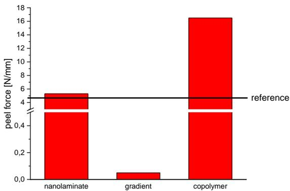
Fig. 5. Peel forces as a function of the different types of coatings.
