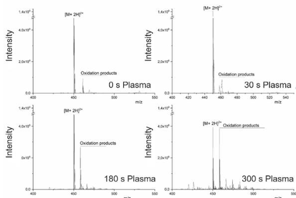
Fig. 2: DI/MS-data of Angiotensin 1-7 treated with the COST-jet for 0-300 s. The intensity is plotted against the mass to charge ratio of observed species.
