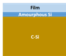
Fig. 4. Illustration of the film thickness on a silicon substrate after plasma deposition
