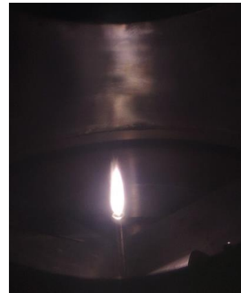
Fig. 2. Photo of the torch sustained by the focused beam of 263 GHz waves.
