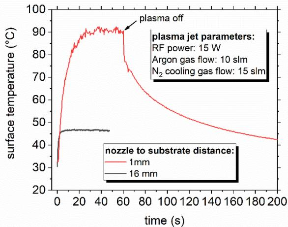
Fig. 4. Measured scaffold temperatures for different nozzle to substrate distances
