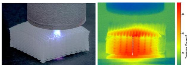
Fig. 2. Plasma jet focussed on a polymer scaffold (left: photo / right: thermal image)
