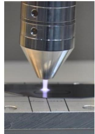
Fig. 1. Used plasma jet setup from Nadir S.r.l.
