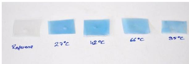
Fig. 8. pp-MAA-VTMOs layers coated at different substrate temperatures stained with methylene blue
