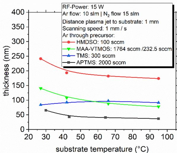
Fig. 5. Layer thickness as a function of substrate temperature for pp-HMDSO, pp-MAA-VTMOS, pp-TMS and pp-APTMS layers
