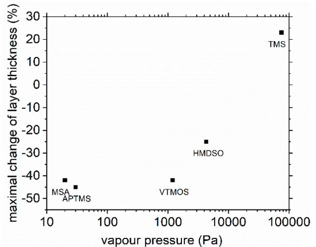
Fig. 6. Correlation between precursor vapour pressure and change of layer thickness
