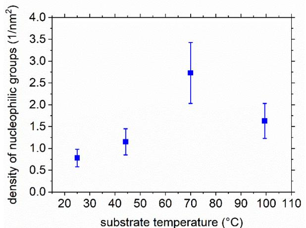
Fig. 7. Density of nucleophilic groups of pp-APTMS layers made with different substrate temperatures
