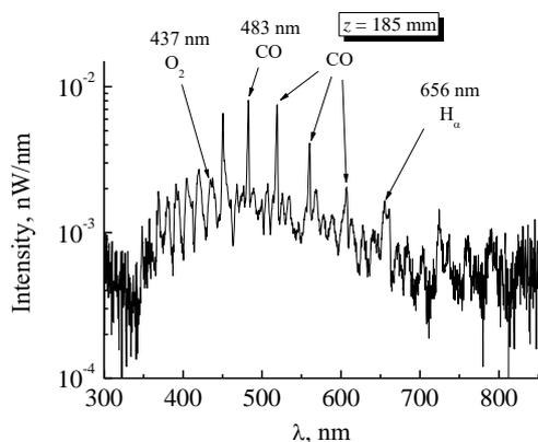
Fig. 3. Spectrum of discharge optical emission in carbon dioxide at distance of 185 mm from the cathode (positive column, maximum glow of the first stratum).
