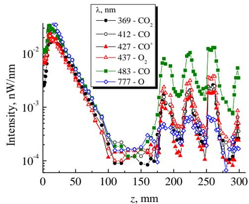
Fig. 4. Photo of the glow discharge in  $\text{CO}_2$  and axial profiles of several characteristic emission lines.
