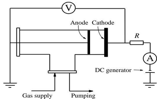
Fig. 1. Scheme of experimental setup.
