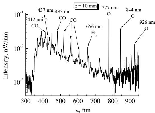
Fig. 2. Optical emission spectrum of the glow discharge in  $\text{CO}_2$  at 10 mm distance from the cathode (negative glow).
