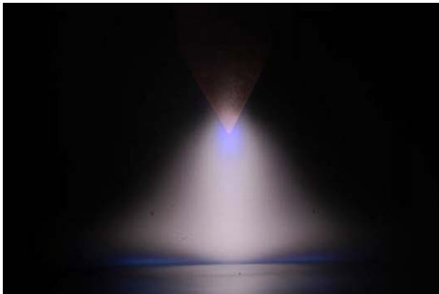
Fig. 5. Photograph of an argon TIG arc with a stainless steel workpiece, for the conditions used in the model.
