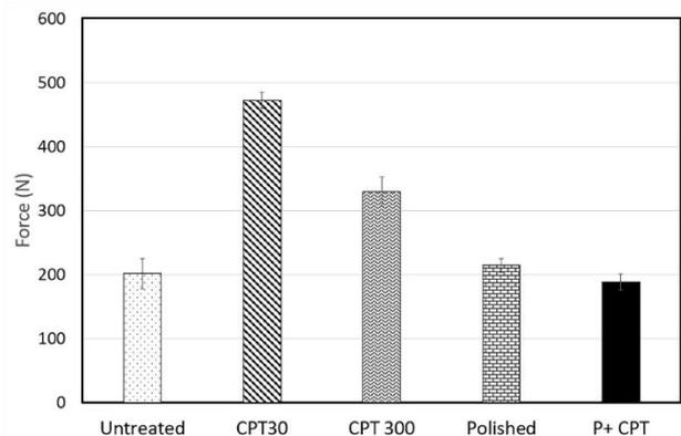
Figure 4: Shearing force required to remove the top 3D printed layer
