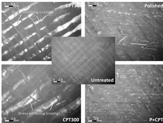
Figure 5: Optical micrographs of the sheared surface for the various treatment conditions
