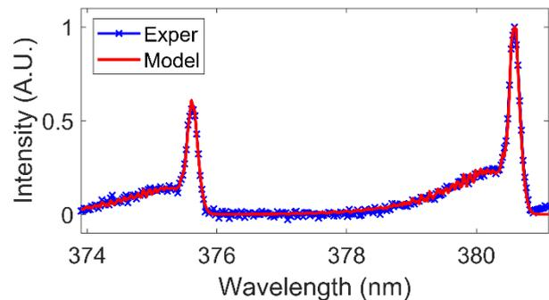
Figure 3: Experimentally measured and SpecAir modelled spectra of the discharge
