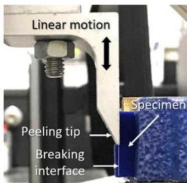
Figure 2: Shear bond strength testing apparatus
