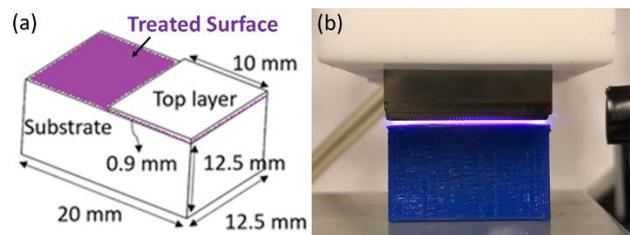
Figure 1: Schematic of the printed part (a) and plasma treating of the part (b)
