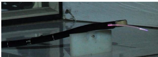
Fig. 8. Cold plasma plume exiting the endoscope
