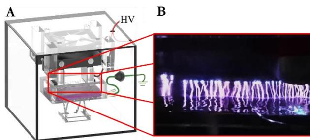
Fig. 1. Multiwire corona plasma source (A) encased in a PMMA box equipped with a fan. (B) Picture of plasma generated by a multiwire corona plasma source on liquid substrate.
