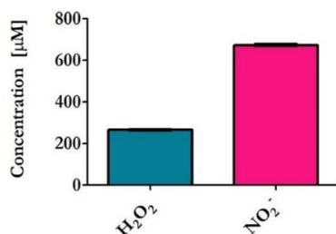
Fig. 2.  $\text{H}_2\text{O}_2$  and  $\text{NO}_2^-$  concentrations of undiluted PAL after 10 min of plasma treatment at PV 18 kV and PRF 1 kHz. The measurements were performed using Amplex<sup>®</sup> Red Hydrogen Peroxide Assay Kit (Thermo Fisher Scientific, Waltham, MA, USA) and Nitrate/Nitrite colorimetric assay (ROCHE, Basel, Switzerland).
