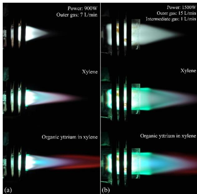
Fig. 3. Comparison of the (a) conical and (b) Fassel torches upon introduction of xylene and organic yttrium dissolved in xylene. The injector inner diameters are 1 mm and 1.2 mm for the conical and Fassel torches, respectively.
