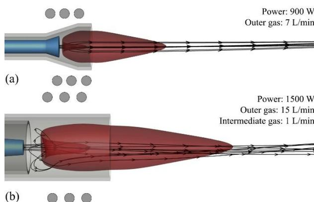
Fig. 2. 3D computer simulations of flow patterns inside the (a) conical and (b) Fassel torches.
