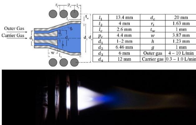
Fig. 1. (Top) Geometrical and operational parameters of the conical torch. (Bottom) Image of the conical torch in
