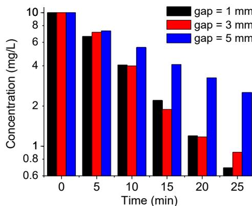
Fig. 5. Time evolution of MB concentration during plasma treatment under three gaps: 1, 3, and 5 mm.
