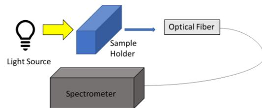
Fig. 2. Schematic of the home-made absorption apparatus to measure degradation rate of methylene blue.
