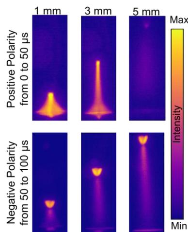
Fig. 4. ICCD images (exposure is 50 $\mu$ s) of the plasma column for three gaps: 1, 3, and 5 mm.
