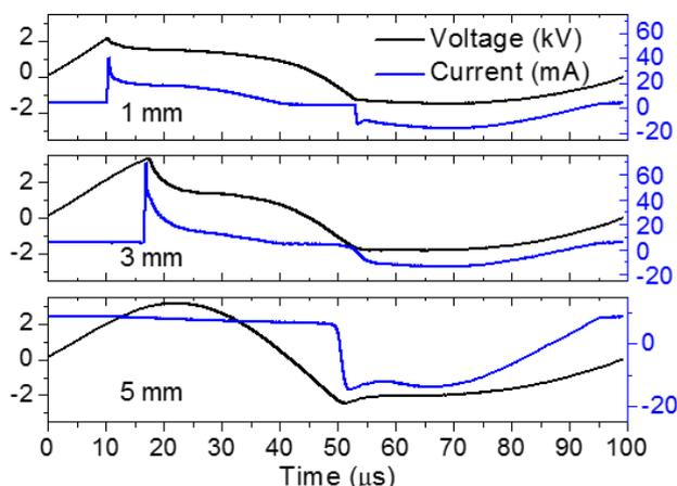
Fig. 3. Typical current and voltage characteristics for three gaps: 1, 3, and 5 mm.
