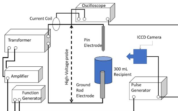
Fig. 1. Schematic of the experimental setup used to generate air plasma in contact with water.
