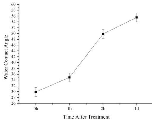
Fig.5. The water contact angles of different time (0h, 1h, 2h,1d) after treated by Ar plasma
