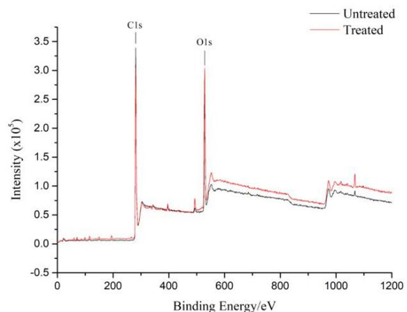
Fig.8. XPS full scan spectra of untreated and treated SMC material to the untreated SMC material. The reason is that the atmospheric pressure Ar plasma consists of high-energy
