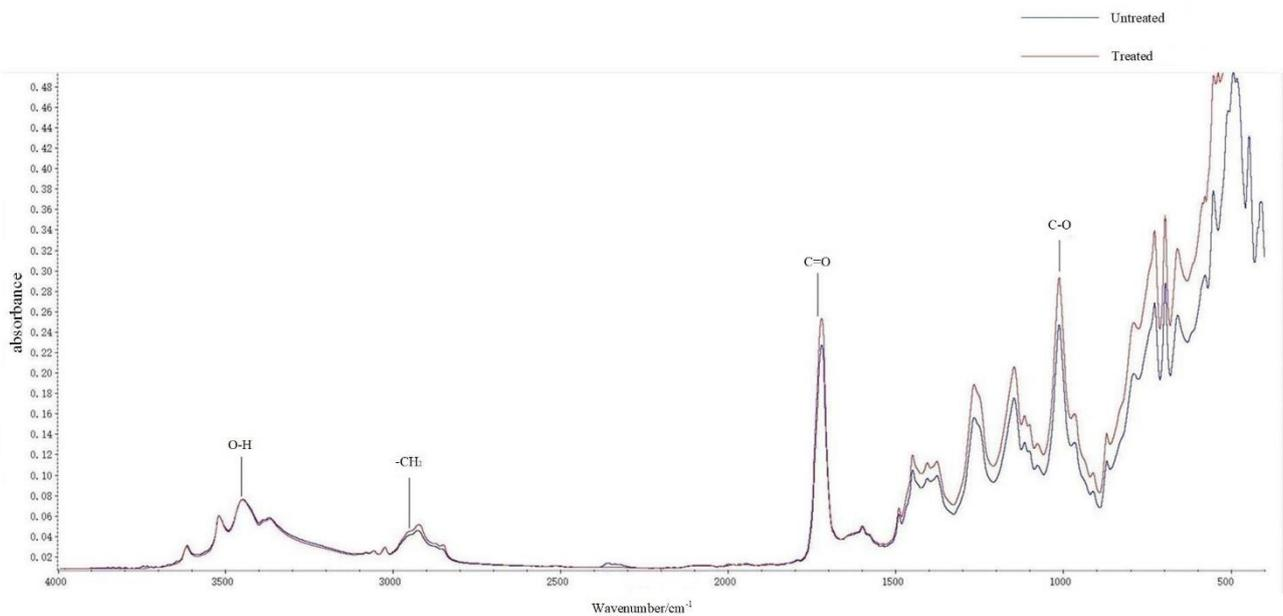
Fig.7. FTIR results of untreated and treated SMC material
