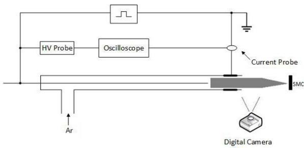
Fig.1. Schematic of APPJ setup.
